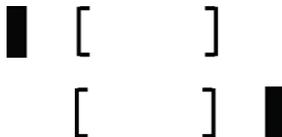
If a left or right arrow appears, then the metal in the sample is most likely not the metal selected.
